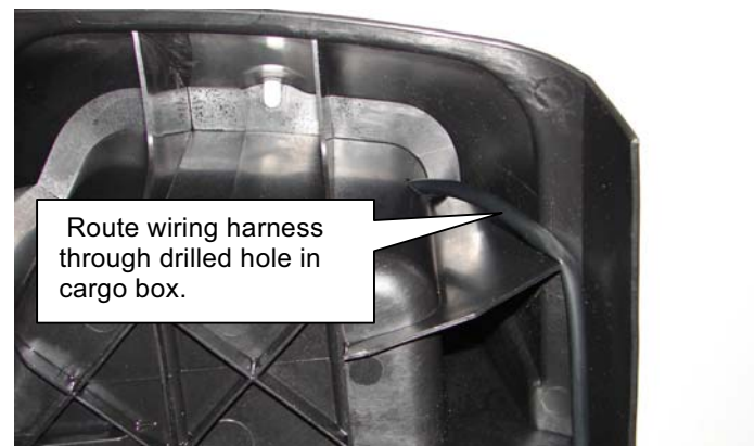
Wiring Harness Routing to Drilled Hole in Cargo Box
