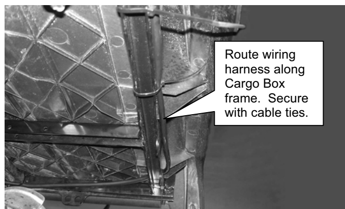
Wiring Harness Routing - under Cargo Box
