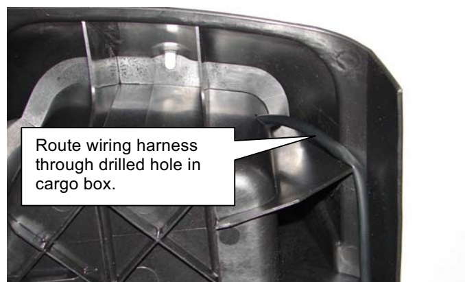
Wiring Harness Routing to Drilled Hole in Cargo Box
